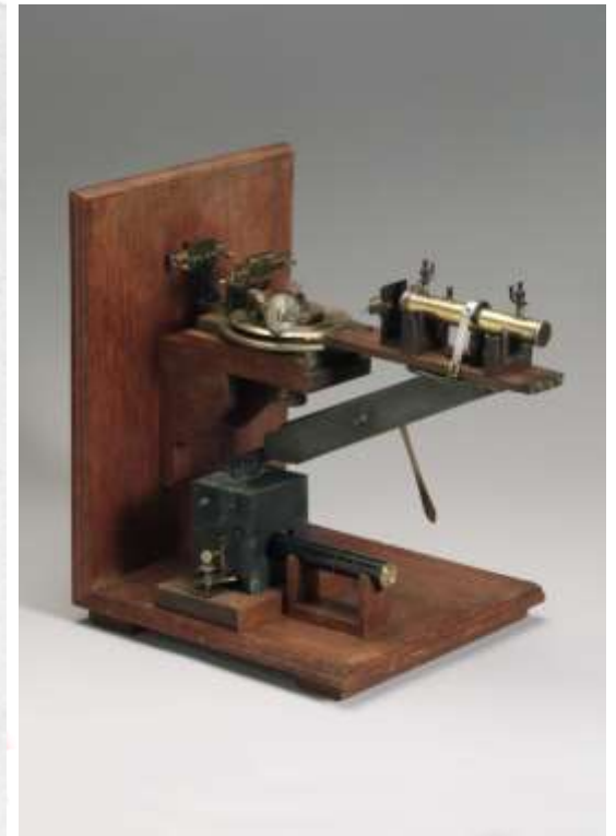
Original Bragg x-ray spectrometer, developed by William Bragg at Leeds University, 1910–1926
